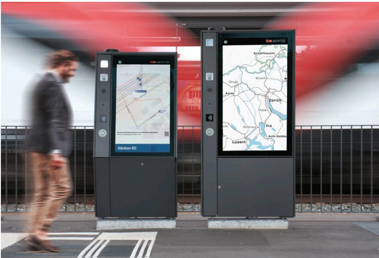
*Digital stiles (smart information displays) of the SBB at Däniken station with network plan and rail replacement plan.*
